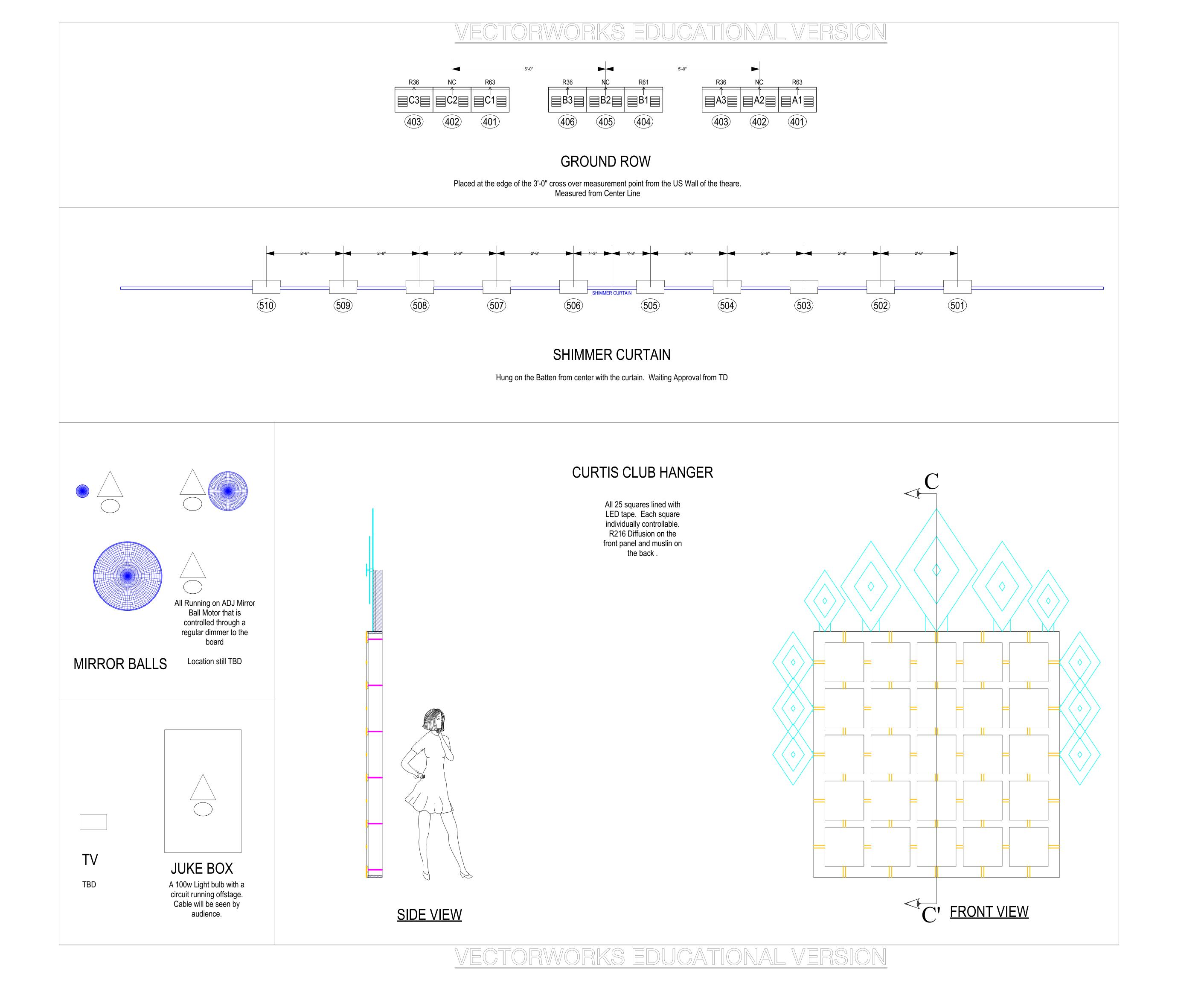
SYMBOLS KEY ETC Source 4 10 Degree ETC Source 4 19 Degree ETC Source 4 26 Degree ETC Source 4 36 Degree Par WFL 18/4? 2/2 2/3 ETC Selador 12/12 2/2 2/2 2/2 2/2 Colortran 30 Degree Colortran Zoom Selecon (Dance) Fresnel Altman Sky CYC Cell Chroma Q Scroller (Rock and Roll Scroll) Apollo Scroller (Stomp Scroll) Wybron Forerunner Scroller (Wybron 2 Scroll) -All lights are on 18" centers unless otherwise noted
