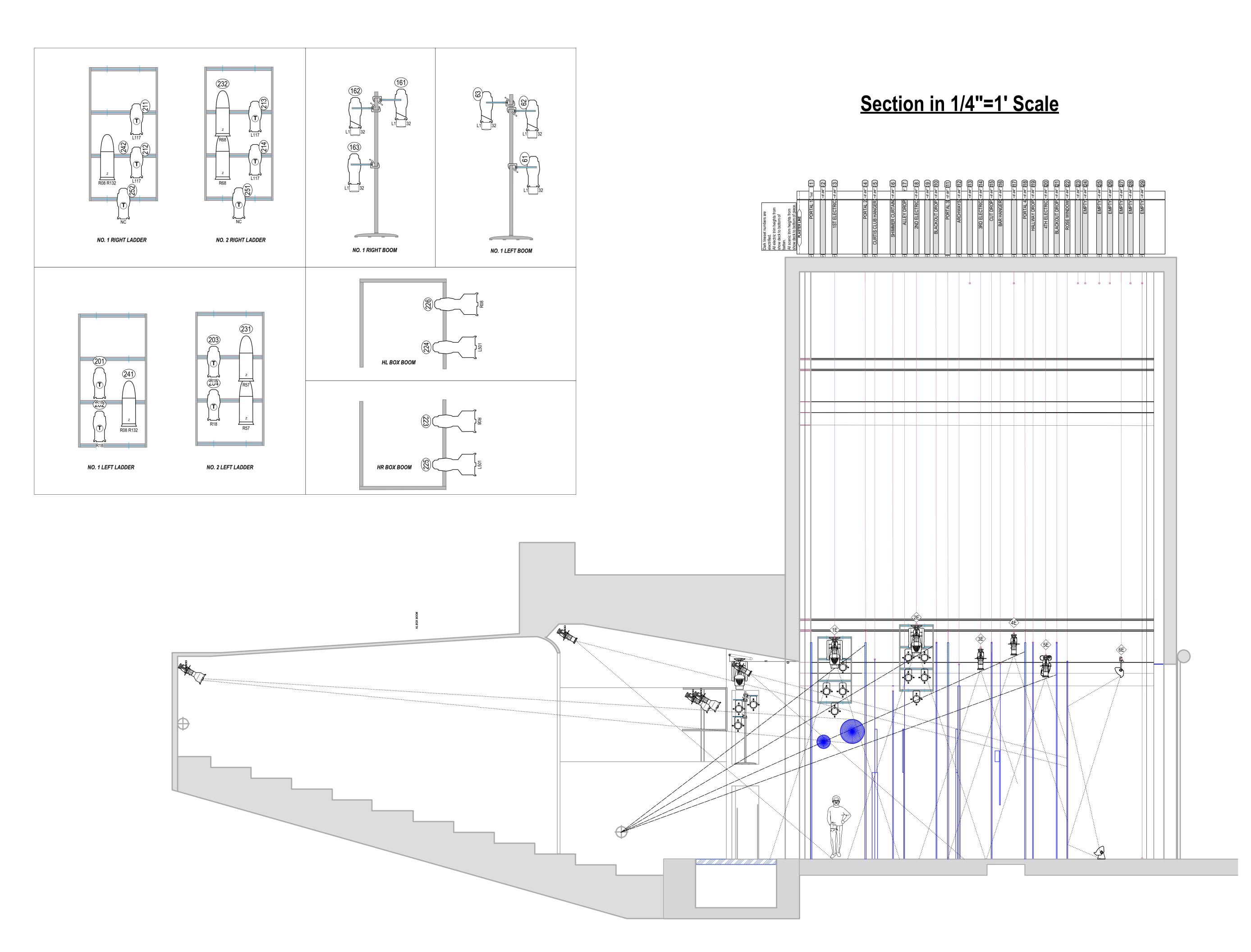
ETC Source 4 10 Degree ETC Source 4 19 Degree ETC Source 4 26 Degree ETC Source 4 36 Degree ETC Selador Colortran 30 Degree Selecon (Dance) Fresnel Chroma Q Scroller (Rock and Roll Scroll) Apollo Scroller (Stomp Scroll) Wybron Forerunner Scroller (Wybron 2 Scroll) -All lights are on 18" centers unless otherwise noted -Practicals are TBD with scenic and lighting designer -Mirror Ball placement is still TBD
